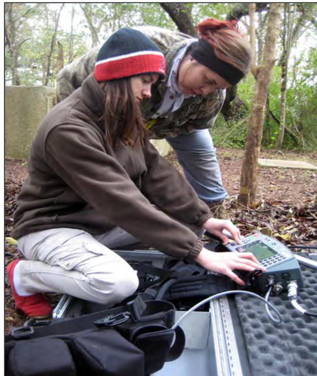
Winter 2014: M. Smith and C. Sheumaker setting up the magnetometer to survey marked cemetery
